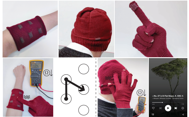
Figure 15: Sleeve-based shape input device and an interactive hat with haptic feedback for music control.
